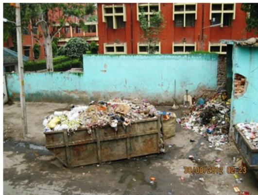
Figure 1: Dhalao (secondary waste collection facility)
